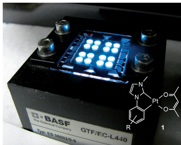
Figure 1. Test diodes based on a new class of emitters: cyclometalated Pt-NHC complexes. [5]
